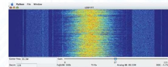
Spectrogram of an FM transmitter with iBOC sidebands.
