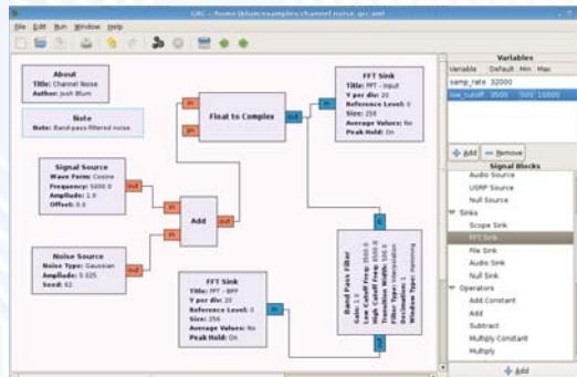
GNU Radio Companion (GRC), a GUI Radio Design system, similar to SimuLink™
